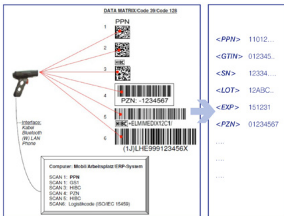
Figure 7: XML-based data exchange between scanner and system
